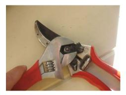
• Remove the spring from the middle of the hand pruner by jiggling it or by pulling it down.
